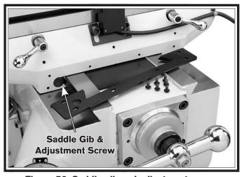
Figure 59. Saddle gib and adjustment screw.
